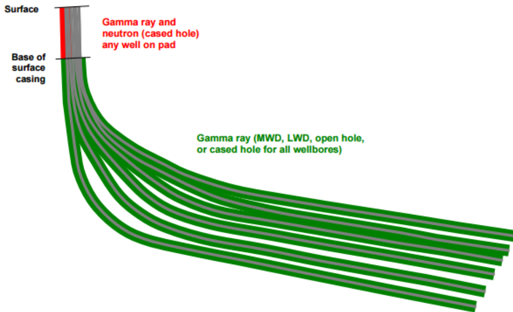
Figure 3 : Site multipuits horizontal (Directive 080, AER)
